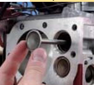
*Are the valves, piston, cylinder or connecting rod damaged?*
